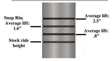
Important: Ensure that the Snap Ring is fully seated in the snap ring groove (you should be able to rotate it manually). Install the spring seat in the orientation shown, making sure the snap ring is fully seated into the groove on the bottom side of the spring perch. Improper installation will cause permanent damage to the shock.
