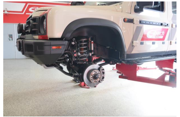
2. Remove both front wheels using 21mm.
